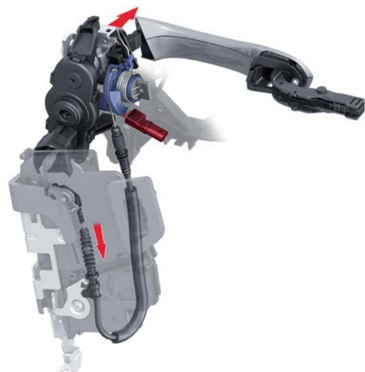
Exterior door operation via a Bowden cable
